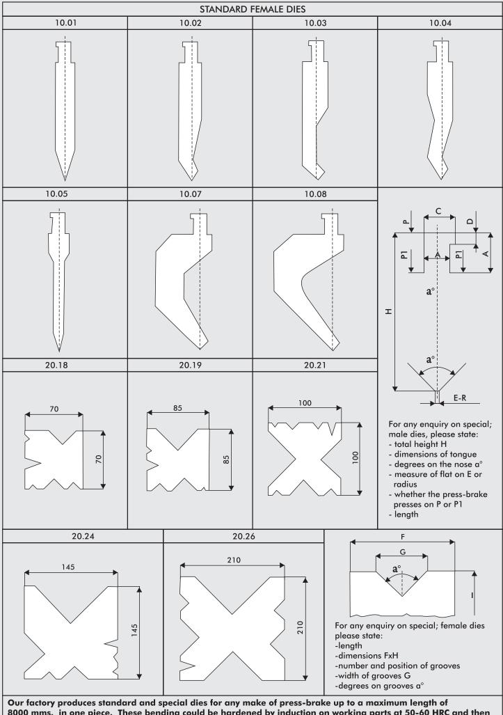
8000 mms. in one piece. These bending could be hardened by induction on working parts at 50-60 HRC and then ground, or from steel with resistance up to 120kg/mm milled, or milled and ground.
