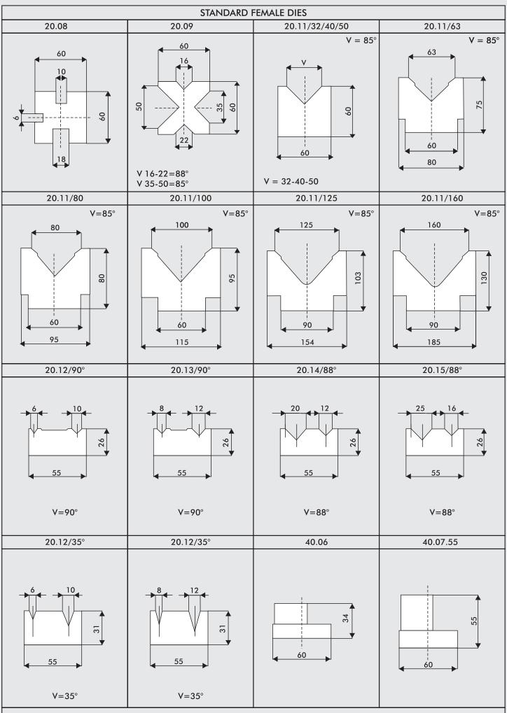
Our standard bending dies are always available in our stock in lengths of mms.: 415, 835 and sectioned. Each bending die is checked very carefully in order to guarantee its QUALITY, PRECISION AND INTERCHANGEABILITY.
