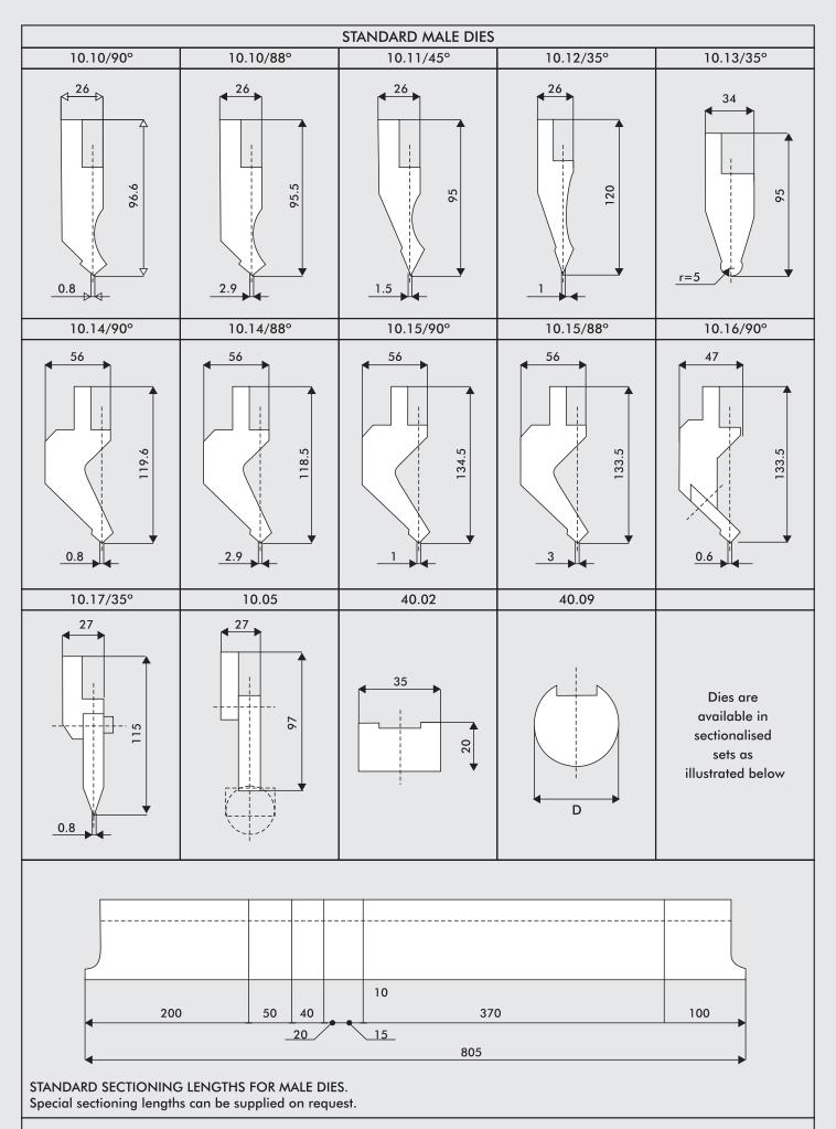
Our dies are made from high steel quality hardened by induction on working parts at 50-60 HRC and then ground with the highest accuracy. We guarantee a perfect matching.
